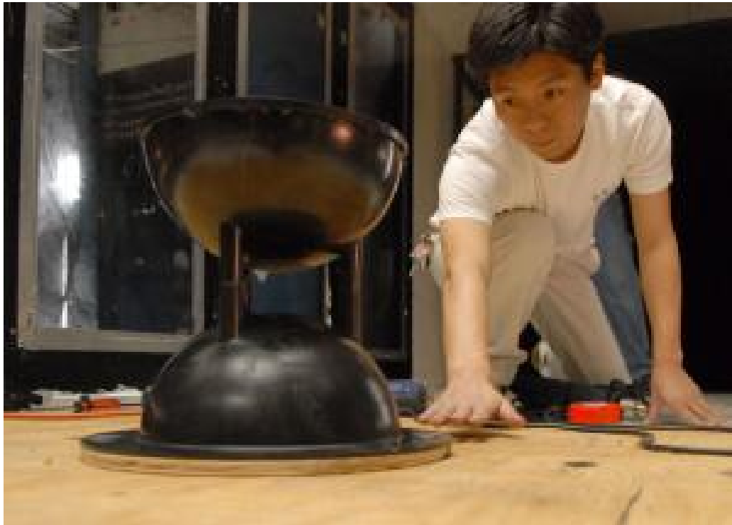
Engineering science and mechanics doctoral student Yihong Yang installs the V2T prototype roof vent in the Virginia Tech stability wind tunnel. (Credit: Photo by Michael Miller, VTIP)
